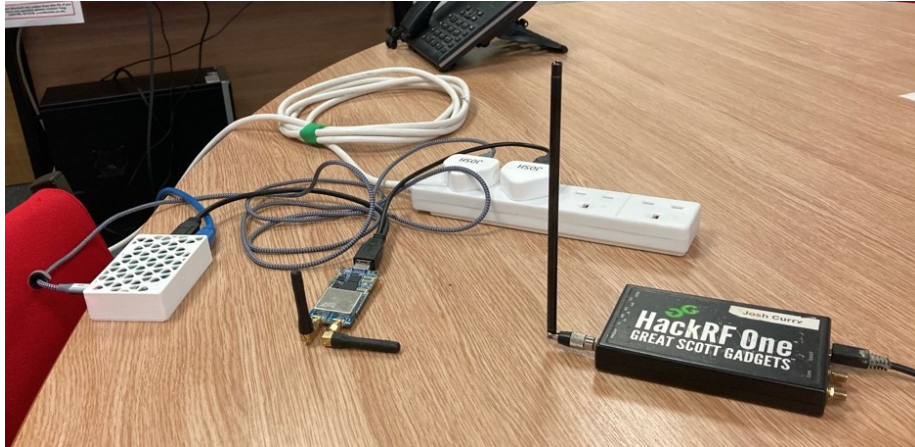
LimeSDR Mini, Raspberry Pi 4 and HackRF One, the latter for spectrum monitoring.
